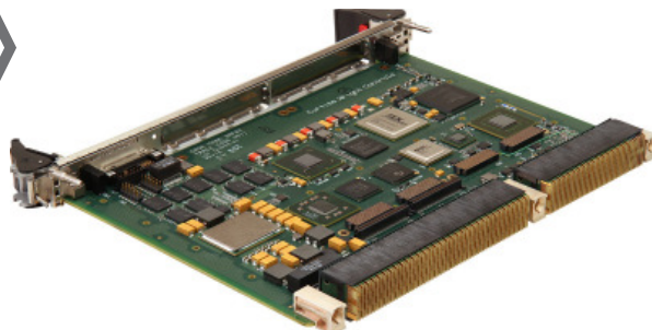
Figure 1 | Curtiss-Wright's VPX6-1958 board, which uses the latest Intel 4th Generation Core i7 processor and dual XMC sites, enable HPEC-Lite systems for SWaP constrained ISR applications.
