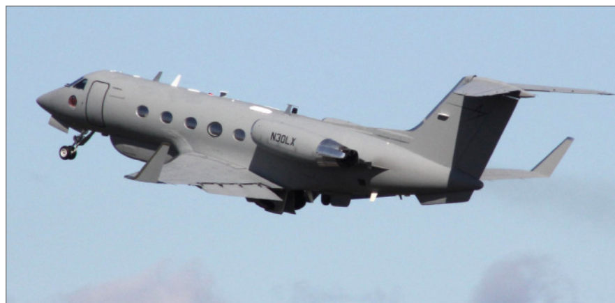
Figure 3 | A flying laboratory, the AML – also known as Dragon Star – is a used business jet that Lockheed Martin engineers modified into a flying test bed for testing and fielding C4ISR capabilities. The Dragon Star configuration addresses requirements for midrange, multi-intelligence platforms such as the Gulfstream III, Havilland D-8, or Beechcraft B350, all of which can be equipped with a variety of sensor and communications systems.
