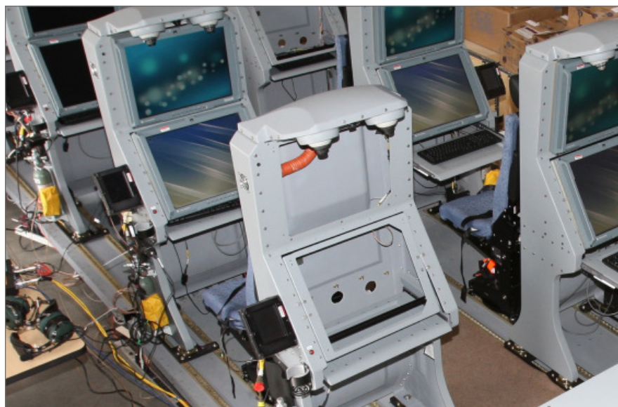
Figure 1 | In Lockheed Martin's palletized Dragon Shield configuration – for users who need to perform multiple missions such as airlift and ISR – the ISR sensor and processing systems are built onto pallets or trailer-like containers that can be rolled on and off aircraft.
